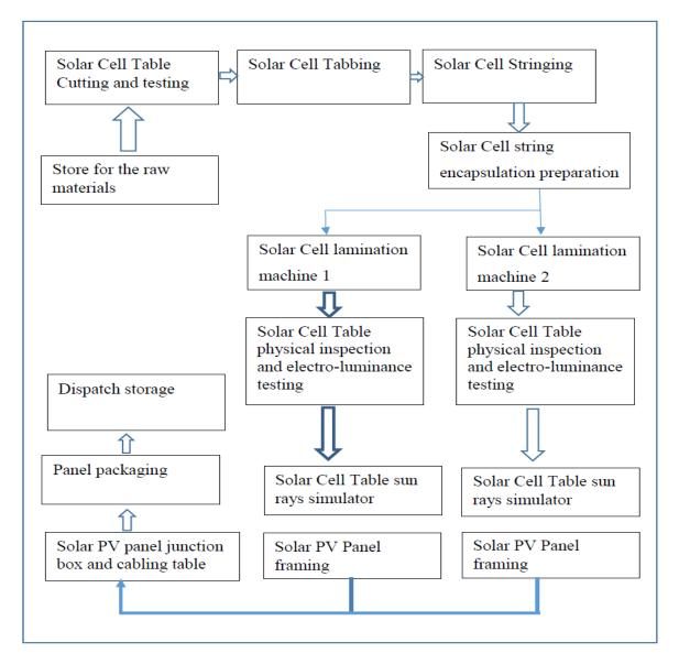
Of importance here is the double or parallel parts (two components) for the solar cell testing & cutting station, the lamination machines, the module inspection and testing machines, and the panel framing stations.
