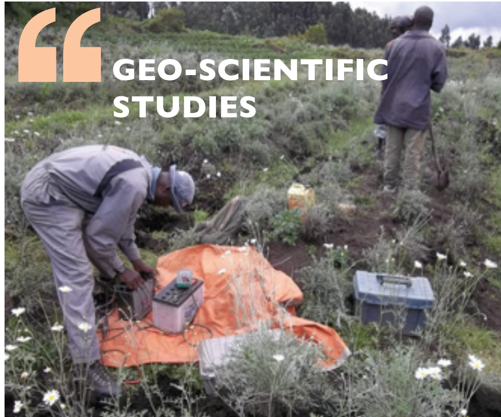
Resistivity Data Collection using MT Equipment
